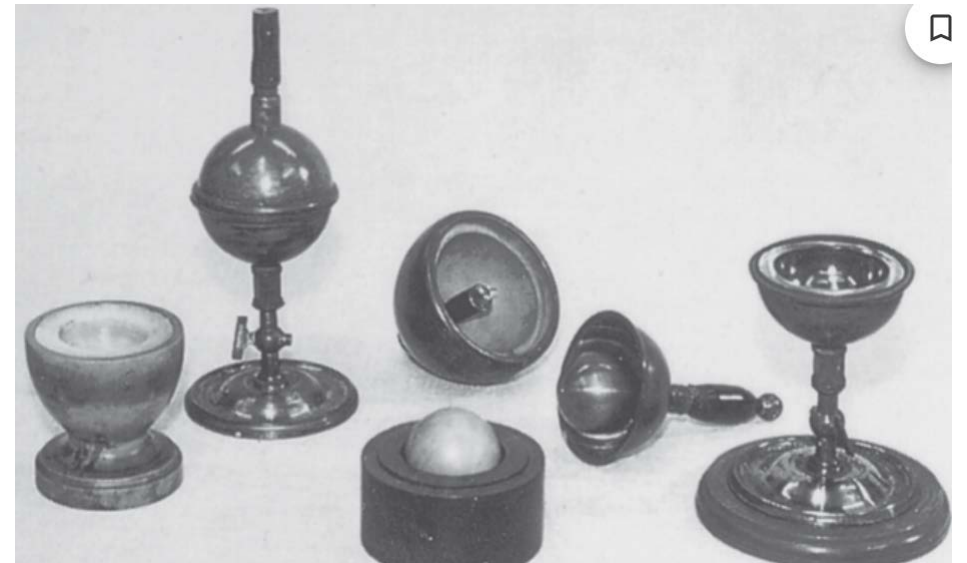
Copyright ©2022 John Wiley & Sons, Inc. Figure 25.5.1 The simple electrostatic apparatus used by Faraday. An assembled apparatus (second from left) forms a spherical capacitor consisting of a central brass ball and a concentric brass shell. Faraday placed dielectric materials in the space between the ball and the shell.
