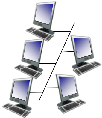
shared wire (e.g., cabled Ethernet)
