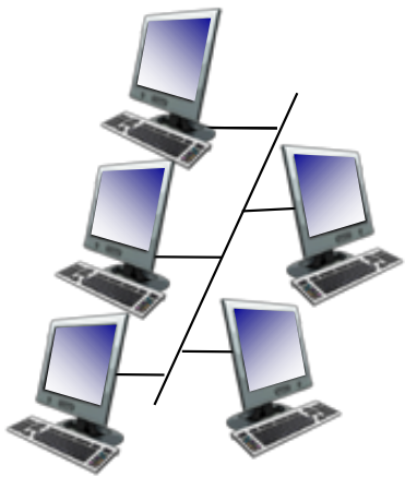
shared wire (e.g., cabled Ethernet)
